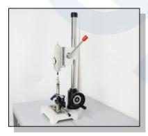
Main machine body to do button test with IMADA PULL GAUGE.
